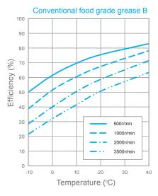
\* CSF-20-100-2A-GR, rated torque
